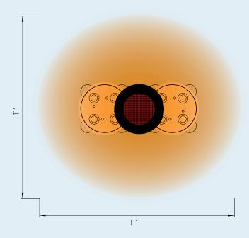
\*HEAT AREA DEPENDENT ON AMBIENT TEMPERATURE AND WIND. OPTIMUM CONDITIONS EXPERIENCED AT APPROX 60°F AND IN A LOW WIND COVERED ENVIRONMENT.
