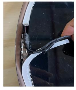
3. Neatly tuck the wiring back into the cavity avoiding pinching or stripping the wires.
