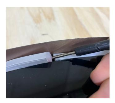
2. Once the end is exposed, carelly pull it out by hand or with long nosed pliers
