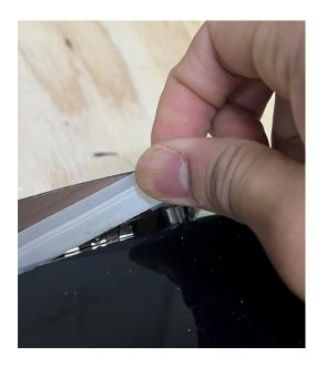
4. Align the new LED strip along the rail, ensuring proper positioning.
