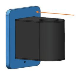
4. Fasten the Wall Bracket Cover using 1 X Dome Head Screw (M4 - Length: 10mm).
