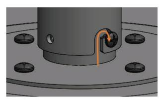
7. Fully insert additional 2 X Dome Head Screws (M4 - Length: 6mm) on both sides, and tighten all four screws, to lock heater in place.
