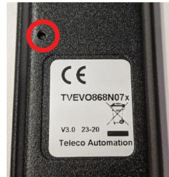
Within 5 seconds of pressing the small button on the rear of the remote, press the small black button on the LED PCB 3 times, holding the button down on the third press. (**2X SHORT PRESS** followed by **1X PRESS & HOLD**)
