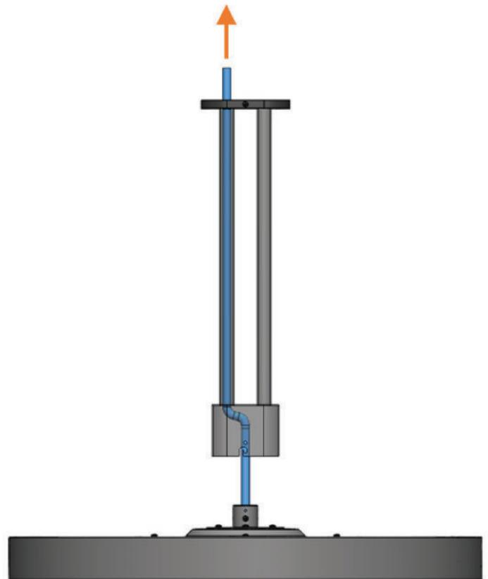
7. Fully insert additional 2 X Dome Head Screws (M4 - Length: 6mm) on both sides, and tighten all four screws, to lock heater in place.
