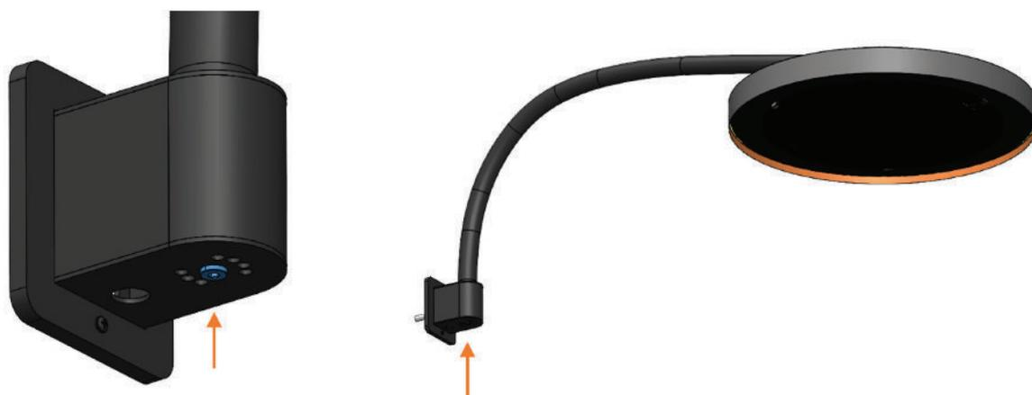
10. Lock the angle of the Wall Mount Pole to the Wall, using 2 X Dome Head Screw (M6 - Length: 10mm). The Wall Bracket angle can be adjusted up to 45° from the wall on each side.
