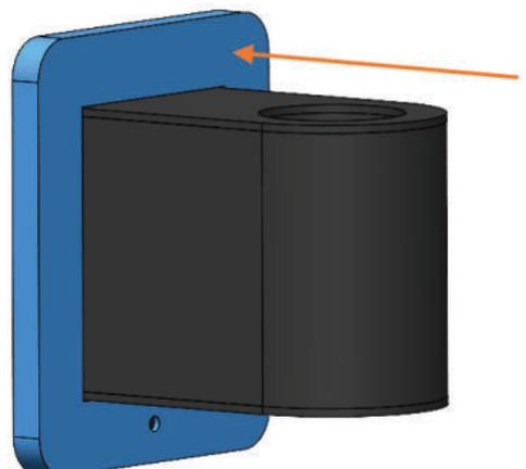
4. Fasten the Wall Bracket Cover using 1 X Dome Head Screw (M4 - Length: 10mm).
