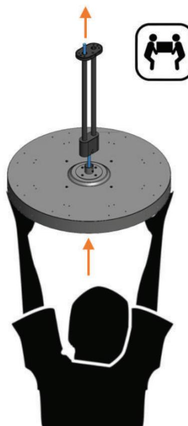
6. Insert the Heater Bracket into the Twin Straight Ceiling Mount Pole by hooking the attached 2X Dome Head Screws (M4 - Length: 6mm) into the slot feature in the Pole.
