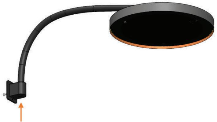
11. If the cable has been routed into the wall cavity, Insert the Cable plug into the optional cable slot.
