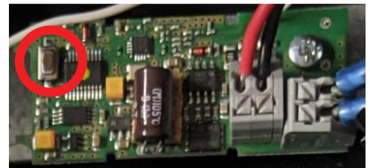
While the LED PCB button is held down, **SHORT PRESS** the **Lights 100%** button on the remote control.
