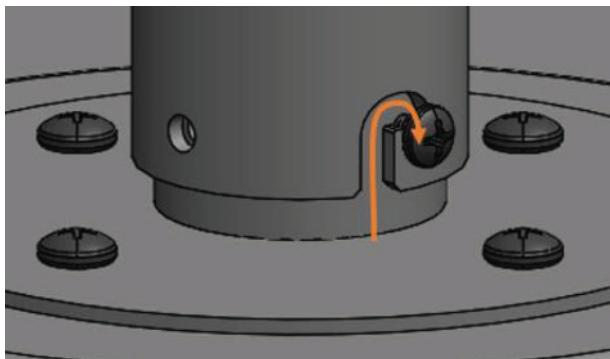
7. Fully insert additional 2 X Dome Head Screws (M4 - Length: 6mm) on both sides, and tighten all four screws, to lock heater in place.
