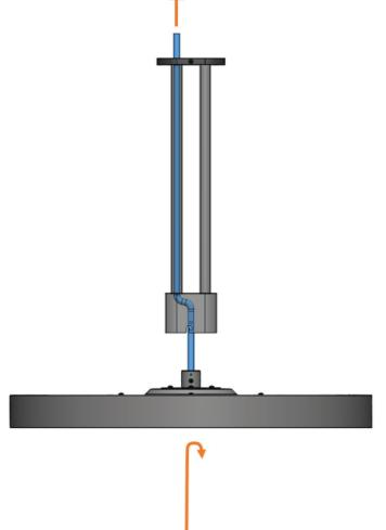
7. Fully insert additional 2 X Dome Head Screws (M4 - Length: 6mm) on both sides, and tighten all four screws, to lock heater in place.
