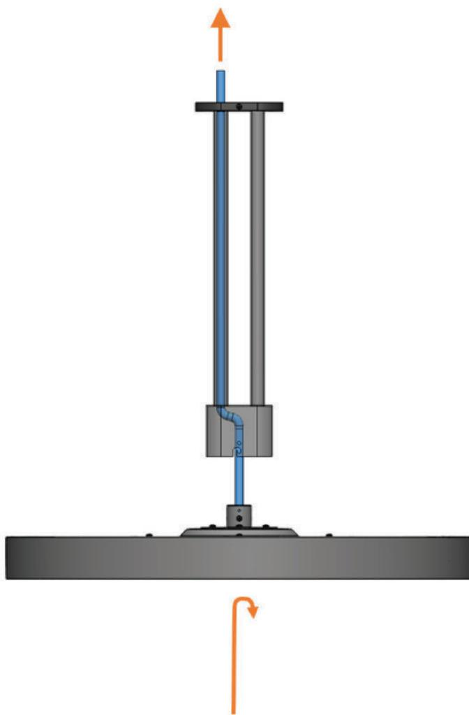
7. Fully insert additional 2 X Dome Head Screws (M4 - Length: 6mm) on both sides, and tighten all four screws, to lock heater in place.
