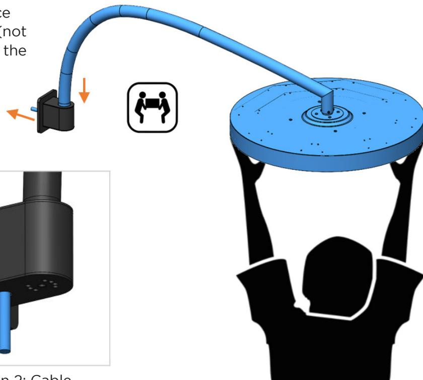
Option 1: Cable into Wall Cavity
