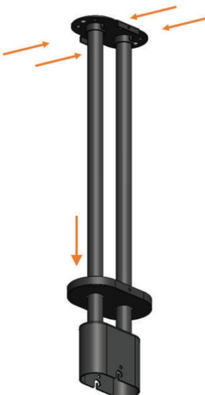
4. Slide the Twin Pole Cap upwards and attach the it to the Twin Pole Roof Bracket using 2 X Dome Head Screws (M4 - Length: 6mm).
