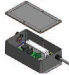
1. Open cover to the Pendant Control Box, by removing 6x Oval head screws (#4-40 - Length: 1/2") from the cover.
