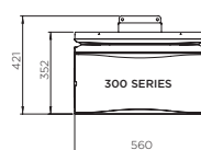
FRONT PROFILE (WITH HEAT DEFLECTOR)
