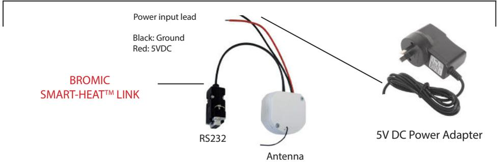
Connect the Bromic Smart-Heat™ Link DB9 to the PC via the COM port or to a USB to RX232 convertor.
